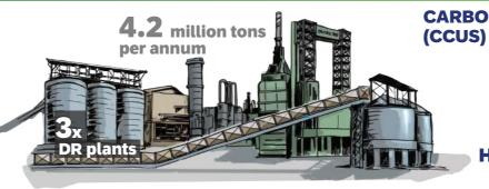
**Natural gas-based** direct reduction process equipped with the **CCUS System (Carbon Capture) and H2 electrolyzer** to produce low carbon footprint compared to other iron melting processes.
